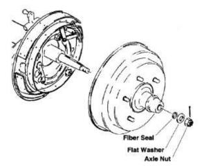
To check it, first remove the cotter key. With the transmission in 1<sup>st</sup> or Reverse gear, and the opposite rear tire on the ground, you can apply a wrench to the axle nut and confirm it is tight.
